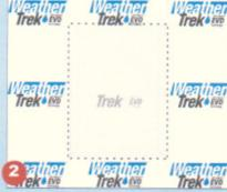
Secure WeatherTrek<sup>nu</sup> firmly in place by fastening it every 12" to 18" along the vertical studs using large-headed or plastic cap nails or minimum 1" crown staples. You may install it over wood based, foam insulative, or fiberboard sheathing, and exterior gypsum board.
